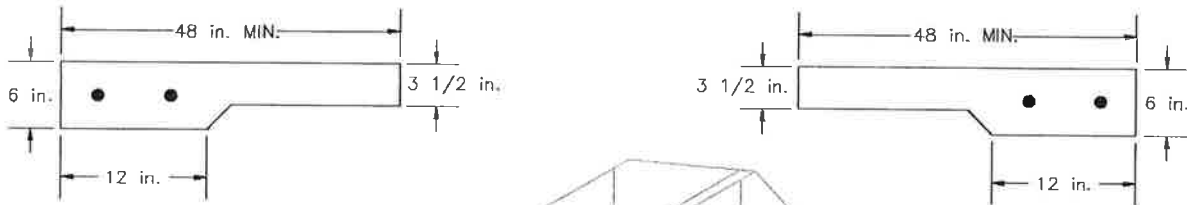
Figure 3-6.2(b) Typical Combined Continuous Concrete Footings (Three-Pad-Pour)
